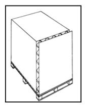
Make height and width dimensions of the faces of the filler material as near as possible the same as the dimensions of the faces of the units they will be separating.
